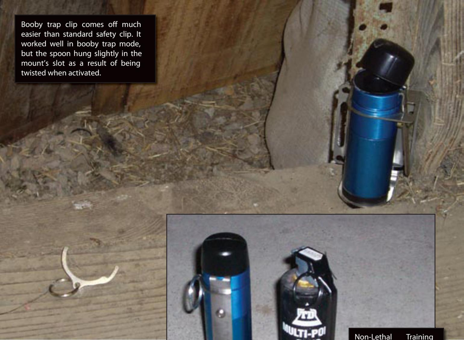
sions of the TG 6 are 1.75 inches in diameter with a height of 6 inches. The total weight is one pound.
